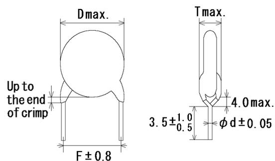
Note) The mark '\*' of lead code differ from lead spacing(F) and lead diameter(d).
