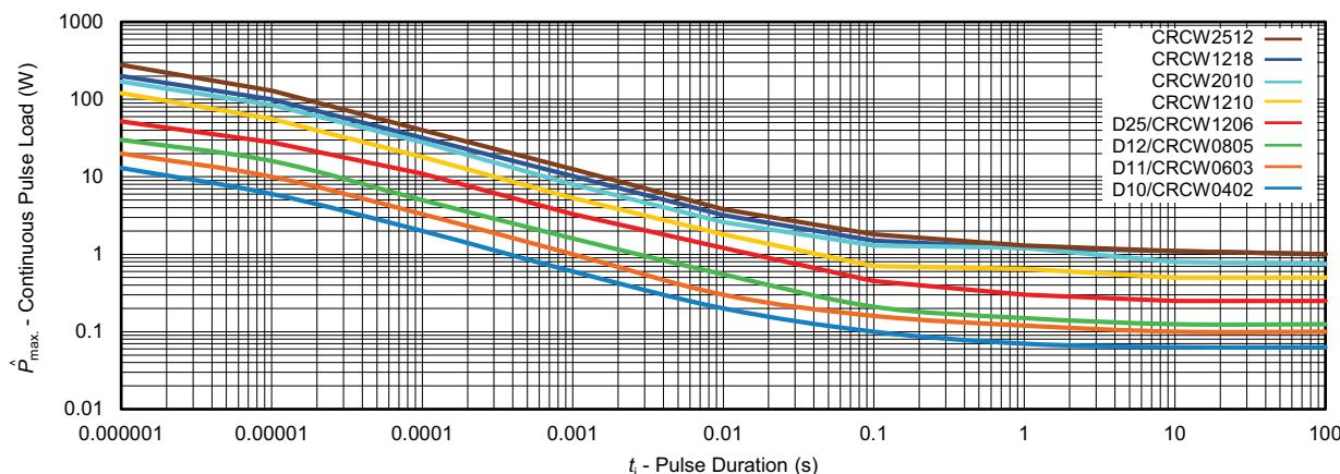
Maximum pulse load, continuous pulses; applicable if  $\bar{P} \leq P(v_{\text{amb}})$  and  $\hat{U} = \hat{U}_{\max.}$ ; standard operation mode, for permissible resistance change equivalent to 8000 h operation
